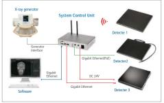
EX) combination of 3 ViVIX models - 1. ViVIX-S Portable, Wireless, 2. ViVIX-S Portable, Wired, 3. ViVIX-S
